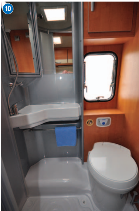
10 The shower head doubles as basin tap and gets in the way. A rigid screen encloses the showering area
